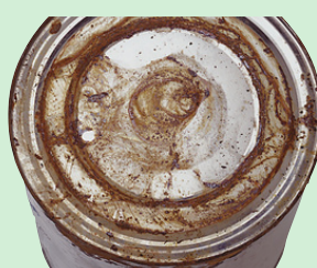
Rust that cannot be wiped off
