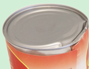
Severe dent in seam
